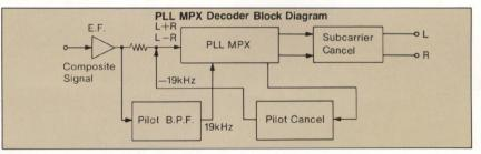
differential switching further enhances the stability of separation, and removes the need for an SCA filter, which could impair audio quality. Use of an IC, rather than discrete parts, for the PLL circuitry makes its performance impervious to temperature and humidity fluctuations, and removes the need for periodic realignment of the MPX stage.
