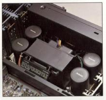
The driver stages for each channel are completely separate, which helps to virtually eliminate transient crosstalk between them. Furthermore, a constant-voltage power supply is used for the pre-driver and initial stages, contributing to stability under highly dynamic transient conditions.
