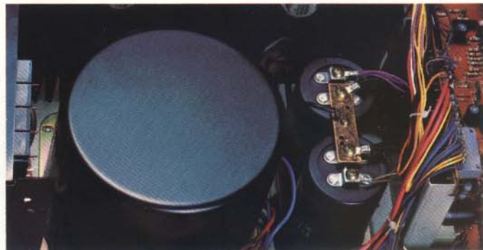
Toroidal-coil transformer and 15,000 \mu F capacitors provide high stability.
