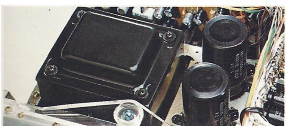
The power section of this receiver is further upgraded by the use in the power supply section of a pair of large 15,000/4F electrolytic capacitors. The SX-750 is the first receiver in its class to use such oversized capacitors, which
